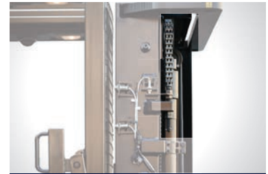
Loose lift chain detection
