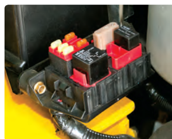
Easy Access to Electric Parts Various electric parts centralized in the dash board provide quick access for troubleshooting.
