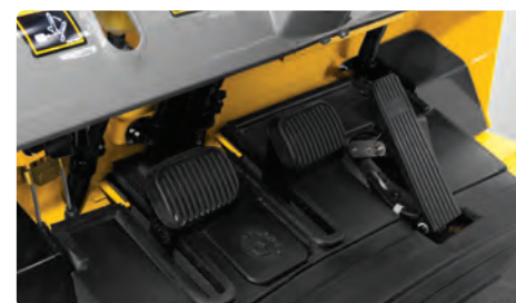
Ergonomically Positioned Pedals Based on human engineering, the accelerator, brake and inching pedals are optimally positioned for convenience while operating the equipment.
