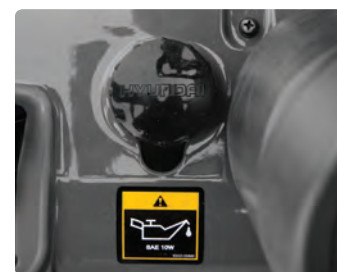
Brake Fluid Reservoir With Level Switch When the brake oil level become lower than Min. level, the warning lamp on the clusters comes on.
