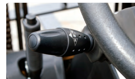
Easy and Safe Shift Lever A single lever on the left side of the steering column gives the operator fast, easy control of direction. The lever must be in the neutral position before the engine can be started.
