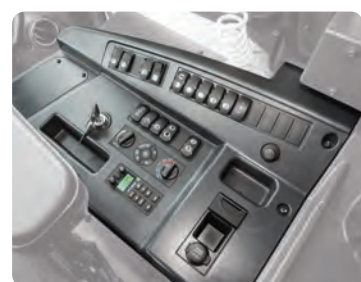
Centralized Instrument Switch Panel
