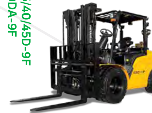
Diesel Forklift 8,000 - 11,000 lbs. capacity
