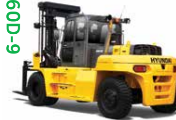
Diesel Forklift 25,000 - 36,000 lbs. capacity
