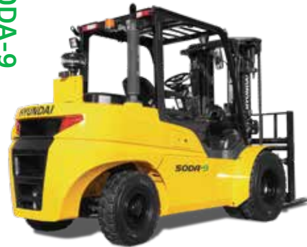
Diesel Forklift 11,000 lbs. capacity
