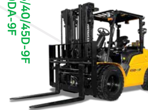
Diesel Forklift 8,000 - 11,000 lbs. capacity
