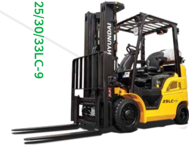
LPG Forklift 5,000 - 6,500 lbs. capacity · Cushion Tire
