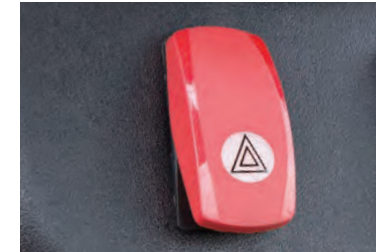
Emergency switch (OPT)
