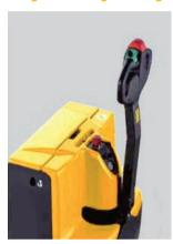
The long tiller design keeps the operator at a safe distance from the truck while working safely and efficiently.
