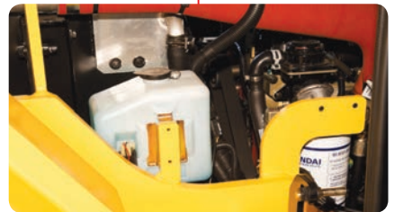
Easy-to-access windshield washer tank
