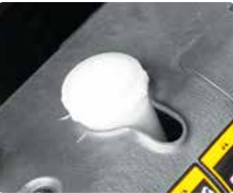
Brake Fluid Reservoir with Level Switch A warning lamp on the cluster is turned on if the brake oil level becomes lower than the required minimum level.
