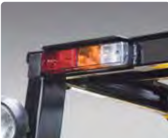
Rear Safety Lamp Rear combination lamps with directional indicators, rear lights and brake lights are positioned for a high level of safety.
